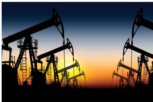
Sucker-rod pumps, colloquially referred to as 'nodding donkeys', are among the most common means of artificial lift for oil wells, particularly in North America where they are familiar to any road traveler. Photo © marrakesh – stock.adobe.com.
